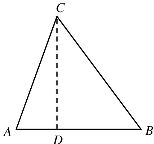
$$\begin{aligned}BC^2 &= (AB - AD)^2 + CD^2 \\&= (AB - AC \cos A)^2 + (AC \sin A)^2 \\&= AB^2 + AC^2 - 2AB \cdot AC \cos A\end{aligned}$$
